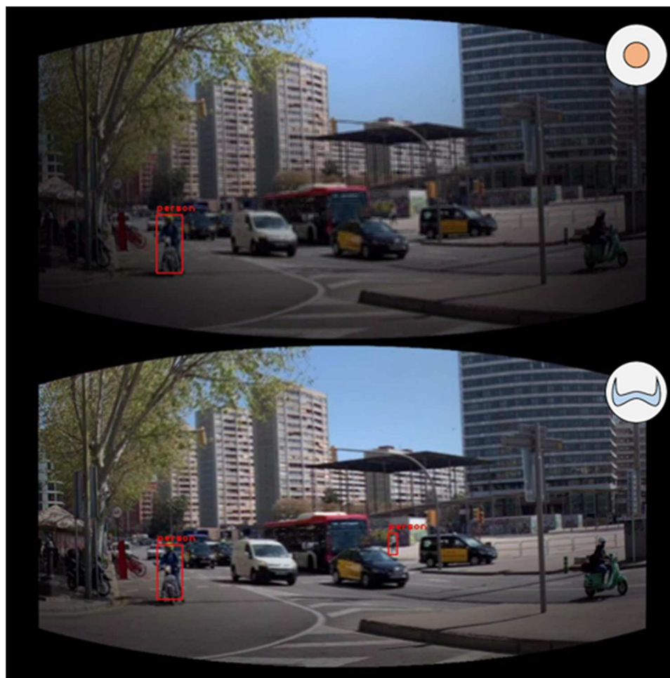
Movie 1. Object detection of the cuttlefish eye-inspired artificial vision system. A dynamic object (i.e., a person on a motorcycle) under uneven illumination is detected on the simulated image sequence of the WPIS and CPIS. A red box appears when the target object is identified with a confidence of >0.8 . The WPIS provides high-contrast imaging, which results in stable object detection.
