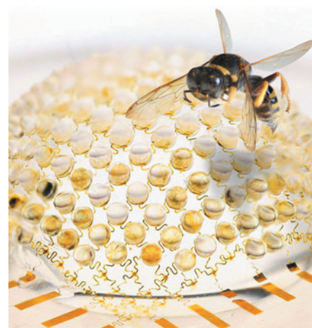
Figure 1 | Insect-inspired visual sensor. Song et al. 1 have designed a visual sensor that resembles, both functionally and structurally, the apposition eye of a daylight insect.
